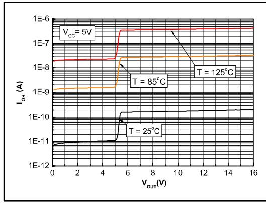
**Figure 8: Output leakage current vs. supply voltage,  $V_{CC} = 5V$**
