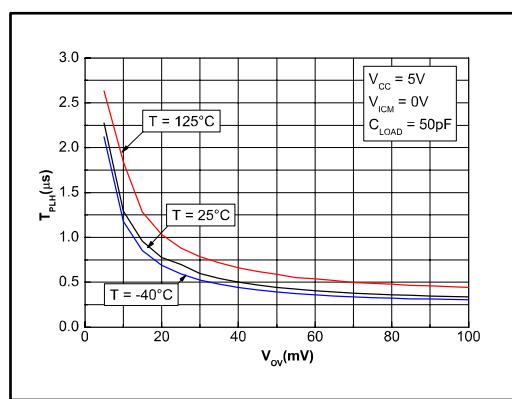
**Figure 14: Propagation delay tPHL vs. input signal overdrive, VCC = 5 V**
