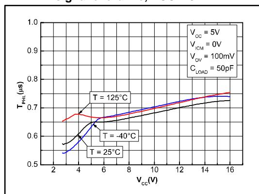
**Figure 16: Propagation delay tPHL vs. supply voltage, VCC = 5 V**
