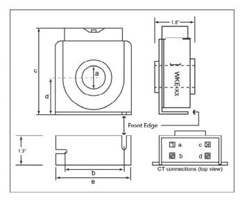
**Primary Current** 2500A **Secondary Current** 350mA NSV 600Vac **BIL Rating** 2000V **Rated Frequency** 10 - 1000Hz
