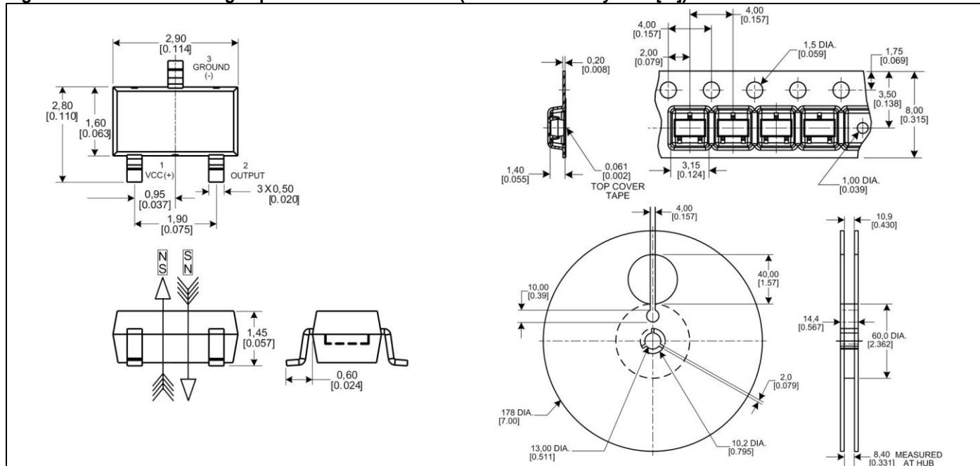
**Figure 6. SS451A Mounting Dimensions (For reference only. mm/[in])**
