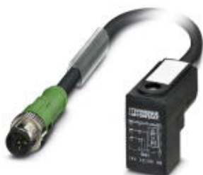
Sensor/actuator cable, 3-position, PUR, black-gray RAL 7021, Plug straight M12, A-coded, on Valve connector C (8 mm), with 1 LED, connected with Z diode, connected with Z diode, cable length: 0.3 m
