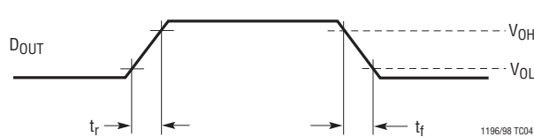
Voltage Waveform for D OUT Rise and Fall Times, t r , t f
