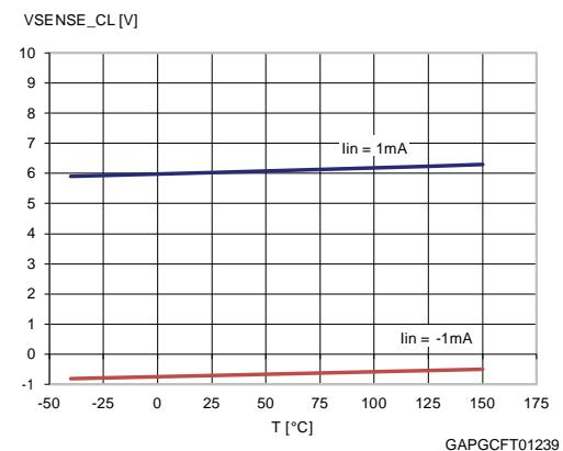
**Figure 29: Vsenseh vs Tcase**
