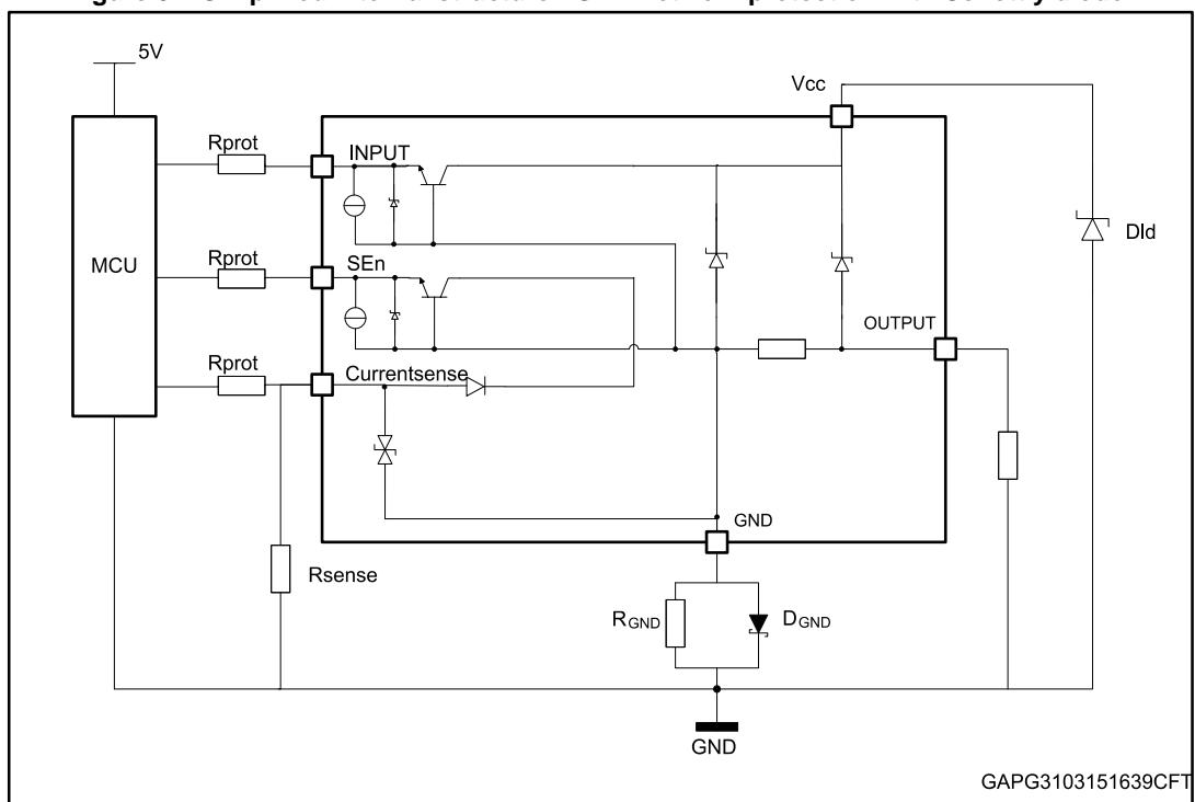
**Figure 32: Simplified internal structure - GND network protection with MOSFET**
