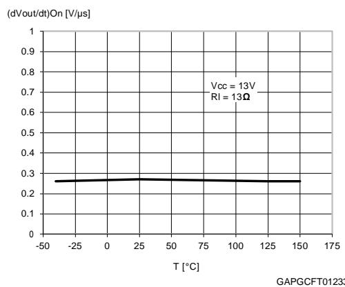
**Figure 23: Turn-off voltage slope**
