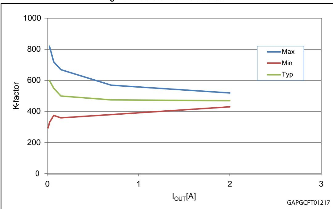
Figure 5: Current sense accuracy versus I<sub>OUT</sub>
