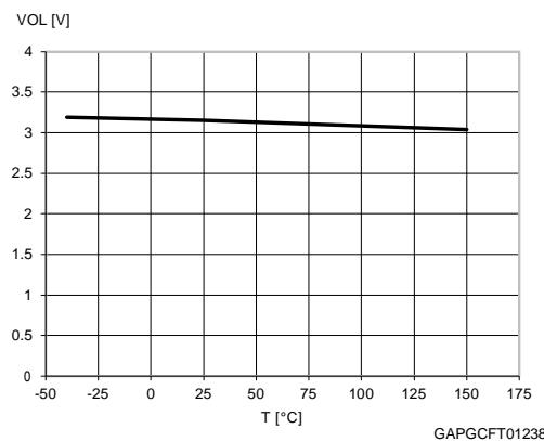
**Figure 28: Vsense clamp vs Tcase**
