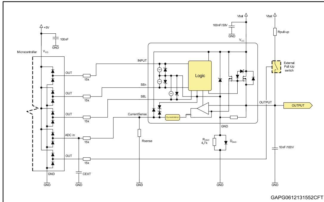
Figure 37: Open-load / short to VCC condition
