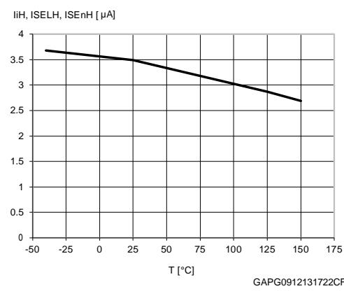
**Figure 17: Low level logic input current**
