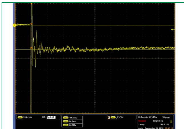
ISO10605 +8 kV Contact ESD Clamping Voltage
