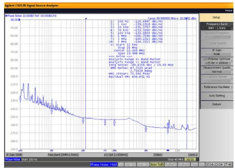
**Figure 2. 553S Output Phase Noise 76fs
