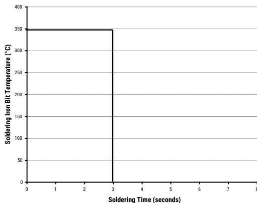
Soldering iron tip temperature should be set at 350°C (+10°C maximum), with the soldering duration not to exceed more than 3 seconds.
