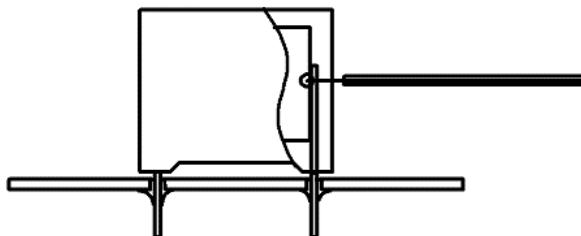
Temperature monitored inside the capacitor.
