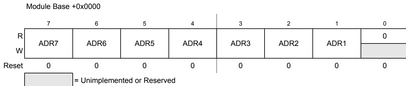
Figure 14-3. IIC Bus Address Register (IBAD)
