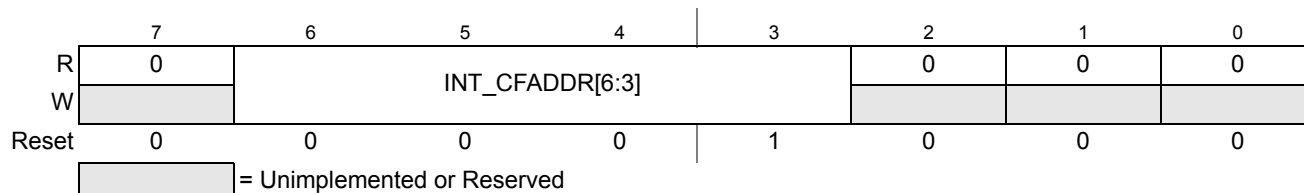
Figure 4-4. Interrupt Configuration Address Register (INT_CFADDR)
