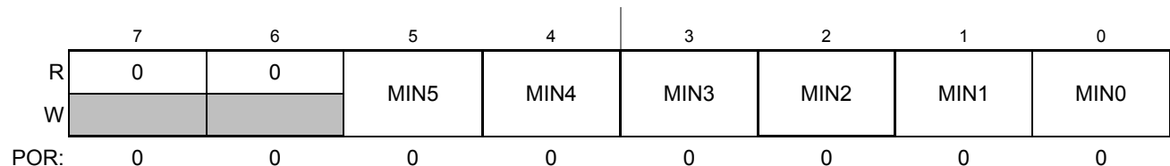
Figure 18-11. Minute Register (MINR)
