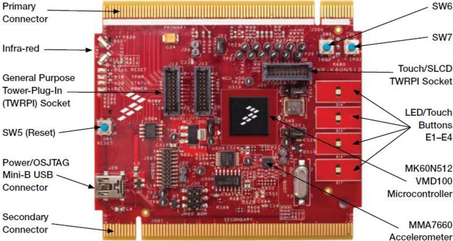
Figure 1: Front side of TWR-K60N512 Module not including TWRPI.
