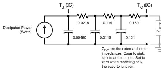
$Z_{EXT}$  are the external thermal impedances: Case to sink, sink to ambient, etc. Set to zero when modeling only the case to junction.
