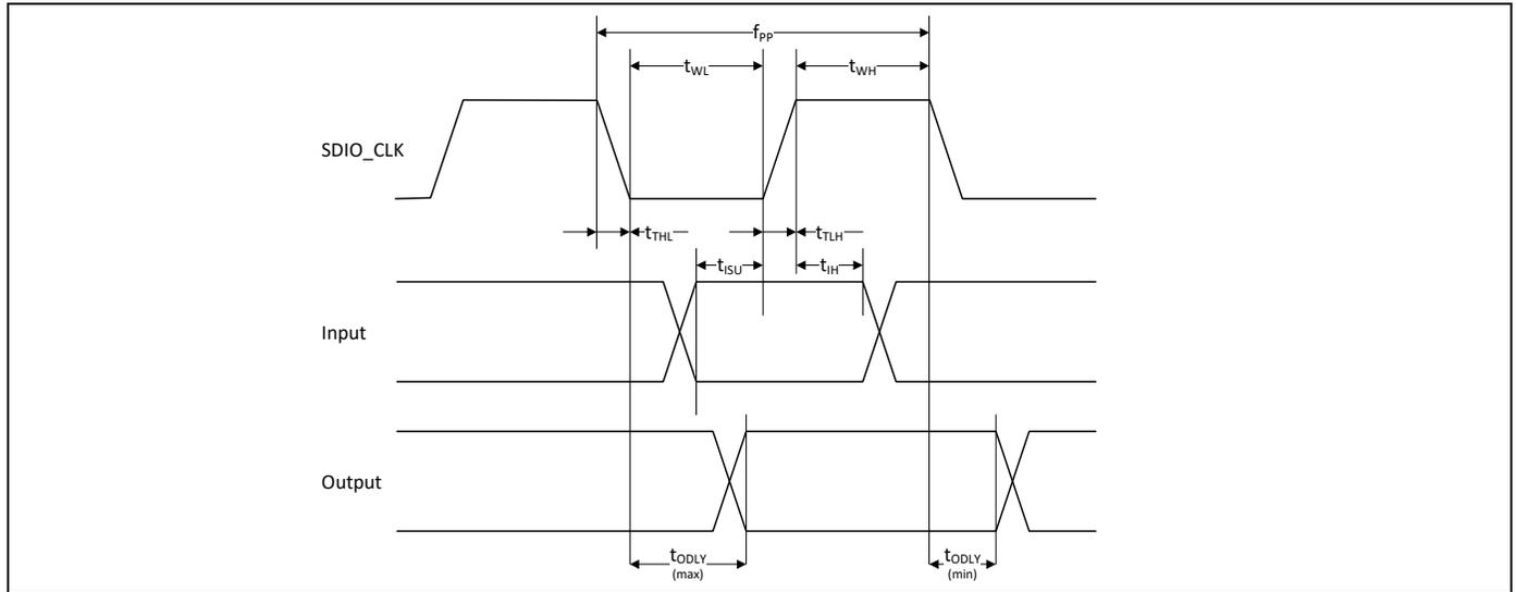
**Table 46. SDIO Bus Timing<sup>a</sup> Parameters (Default-Speed Mode)**
