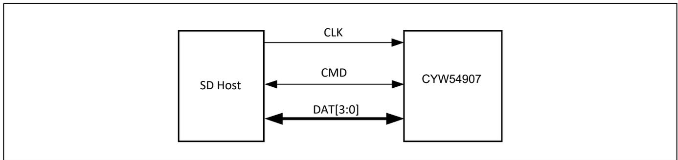
**Figure 7. Signal Connections to an SDIO Host (SD 1-Bit Mode)**
