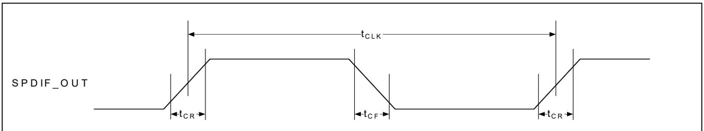
Table 51 provides the S/PDIF biphas mark code timing parameters (to be used in conjunction with Figure 29).
