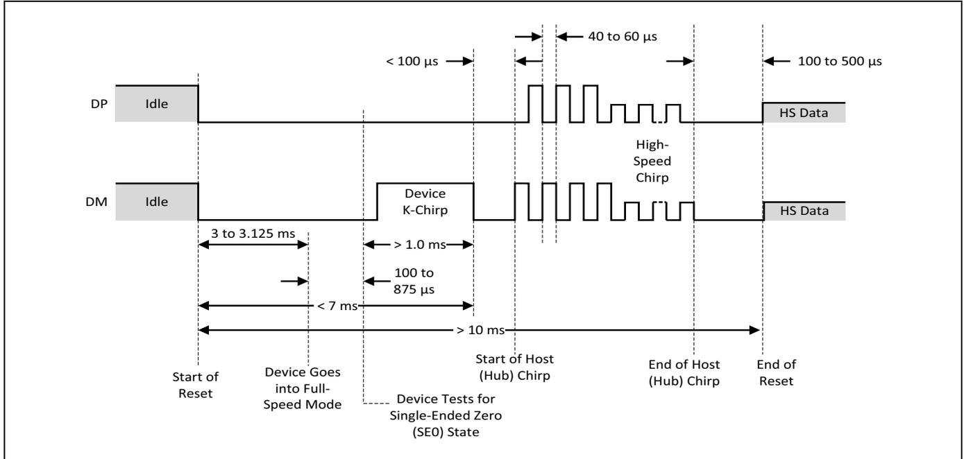
Figure 36 shows the USB 2.0 HS Mode transmit timing.
