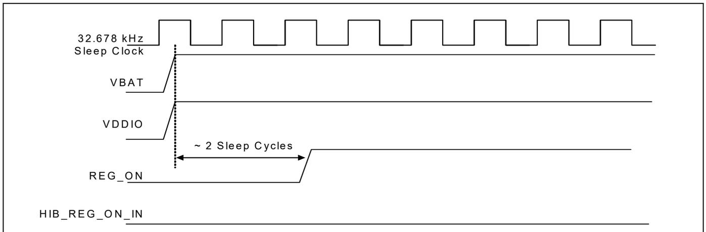
**Figure 39. HIB\_REG\_ON\_IN = High, HIB\_REG\_ON\_OUT Connected to REG\_ON**
