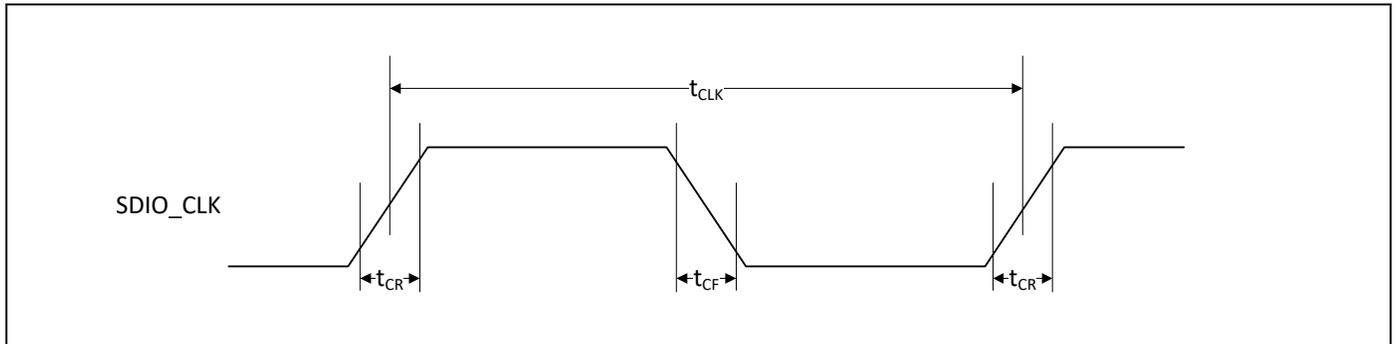
**Table 48. SDIO Bus Clock Timing Parameters (SDR Modes)**
