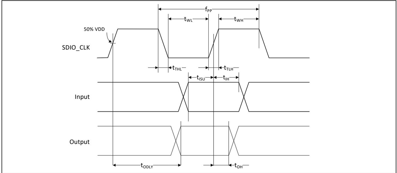
**Table 47. SDIO Bus Timing<sup>a</sup> Parameters (High-Speed Mode)**
