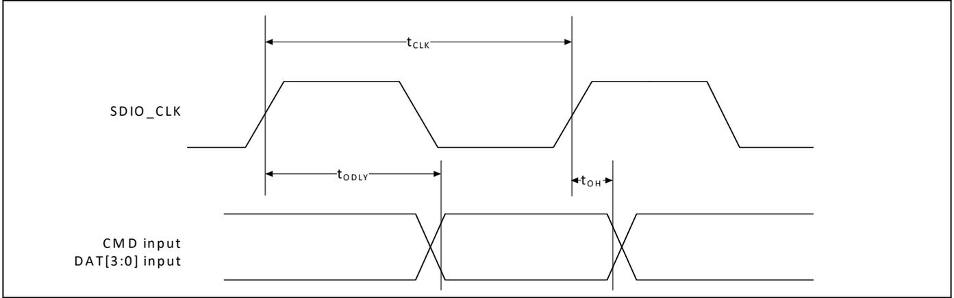
**Table 50. SDIO Bus Output Timing Parameters (SDR Modes up to 50 MHz)**
