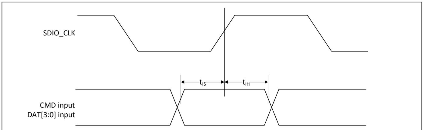
**Table 49. SDIO Bus Input Timing Parameters (SDR Modes)**
