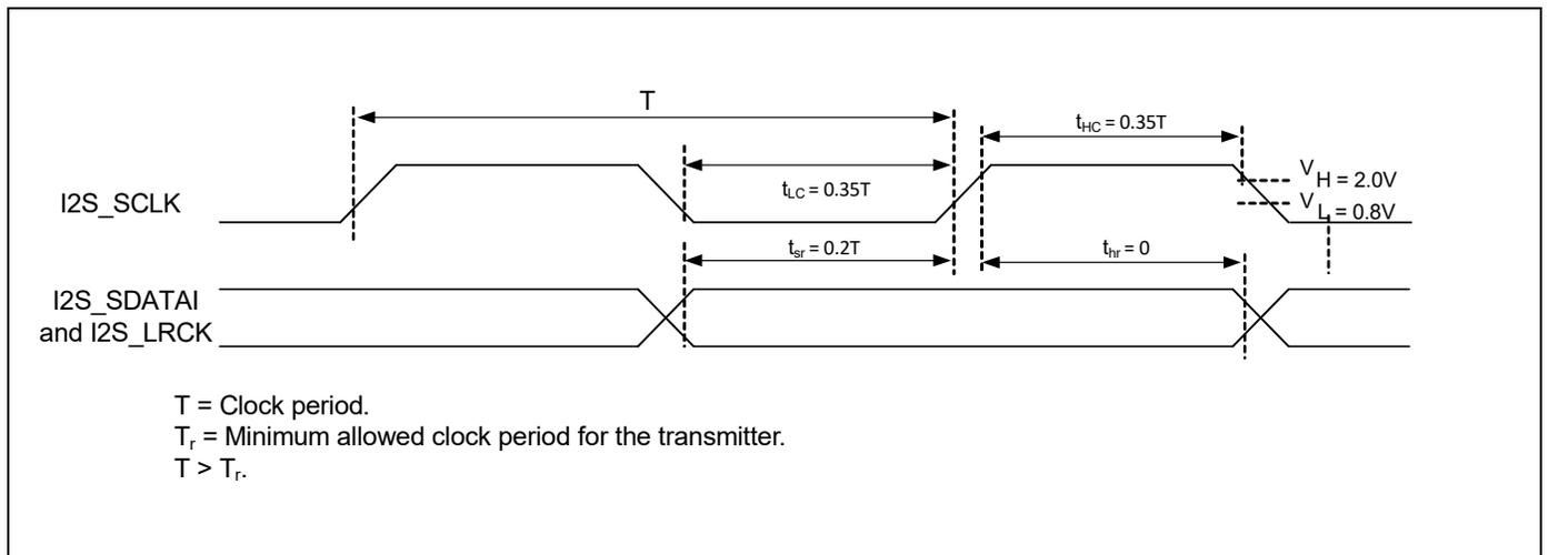
**Table 44. Timing for I<sup>2</sup>S Transmitters and Receivers**
