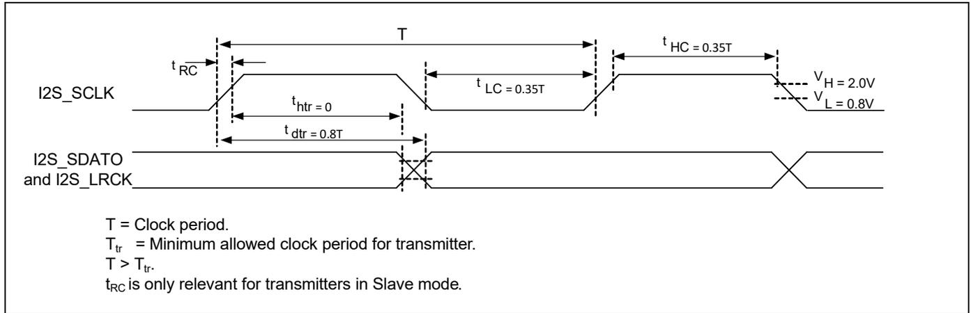
Figure 21 and Table 44 provide the I<sup>2</sup>S Slave mode receiver timing.
