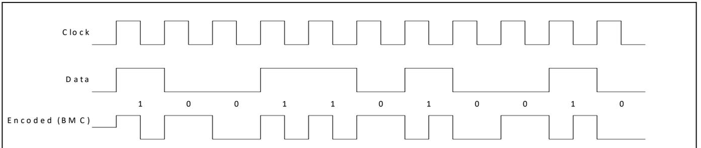
Figure 29 shows the S/PDIF data output timing.
