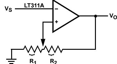
$$V_{UL} = \left\{ \frac{R_1}{R_1 + R_2} \right\} V_O(\text{max})$$
