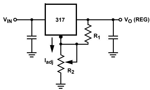
$$V_O(\text{REG}) = 1.25V \left(1 + \frac{R_2}{R_1}\right) + I_{\text{adj}} R_2$$
