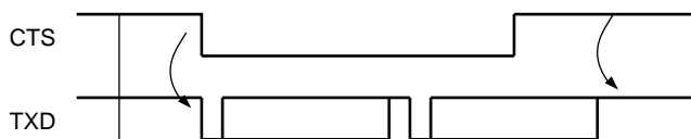
Figure 31-19. Transmitter Behavior when Operating with Hardware Handshaking
