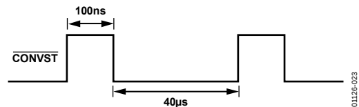
Figure 21. CONVST When Temperature Channel Selected
