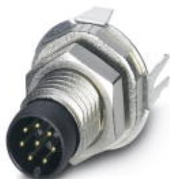
Sensor/actuator flush-type plug-in connector, plug, 8-pos., M8, rear/screw mounting with M8 fastening thread, with straight solder connection
