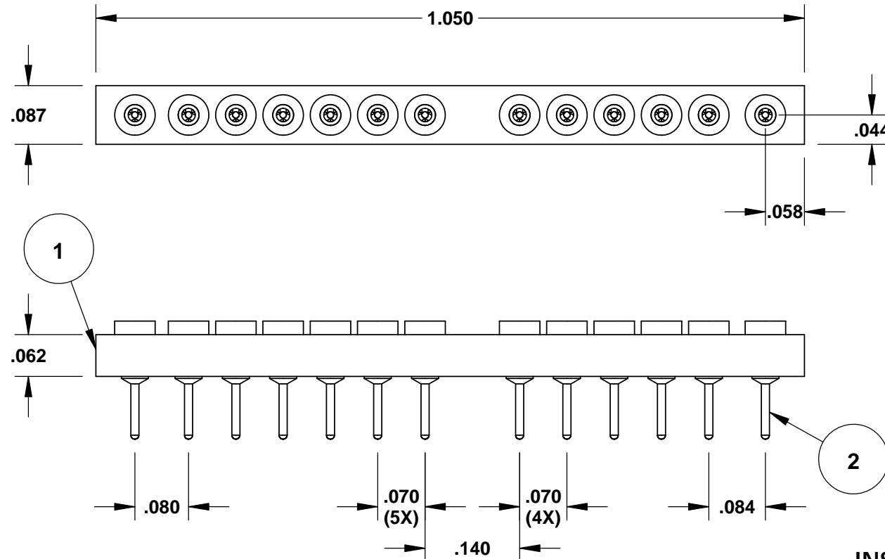
**INSULATOR HOLE DIAMETERS ARE .042"**
