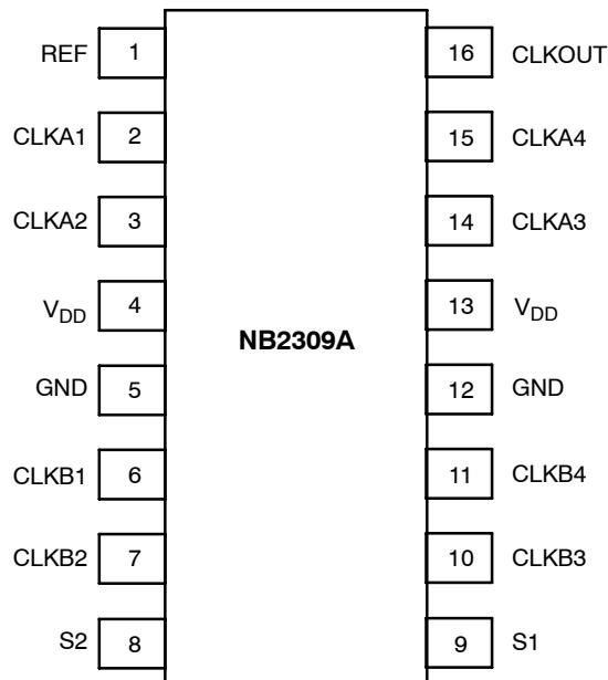
**Figure 2. Pin Configuration**
