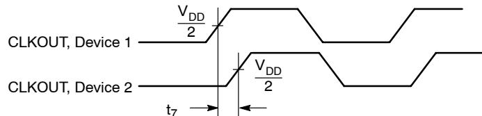
**Figure 7. Device – Device Skew**
