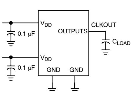
**Figure 8. Test Circuit #1**
