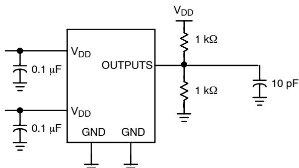
**Figure 9. Test Circuit #2**
