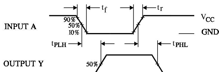
Figure 1. Switching Waveforms
