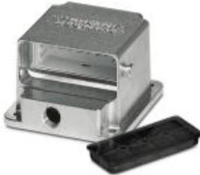
Connector on motor side, EMC metal housing attachment incl. crimp contact insert, with flat seal and coated protective cover, without crimp contacts, housing with coatable thick-layer passivation
