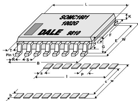
**SOLDER PAD DIMENSIONS** in millimeters
