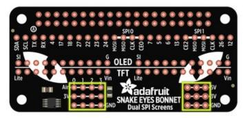
At the bottom-right of the bonnet are a few extra connection points for **5 Volts**, **3.3 Volts** and **ground**, if you have a circuit that needs them. These are OK for **small loads** like ICs or a few LEDs, but *not* for big things like servos, which will need their own power source.
