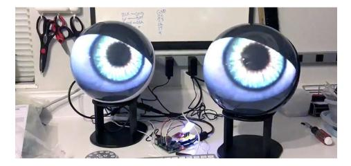
In order to work with the WorldEye display (or other HDMI devices), the code and graphics for this version are slightly different. The TFT/OLED code (eyes.py), designed for two separate physically-wired screens, provides a **distinct shape** for the left and right eyes to approximate the *caruncle* (the inner corner of the eyes). The HDMI code (cyclops.py) generates a single **symmetrical** eye (no carnucle), so it can be fed to an HDMI splitter and not look lopsided on two screens.
