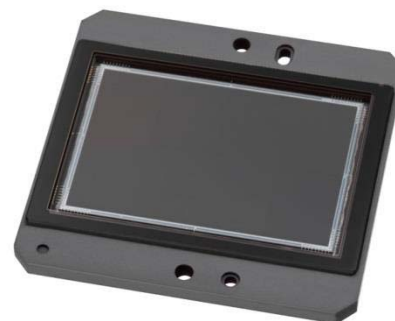
Figure 1. KAI-29050 CCD Image Sensor
