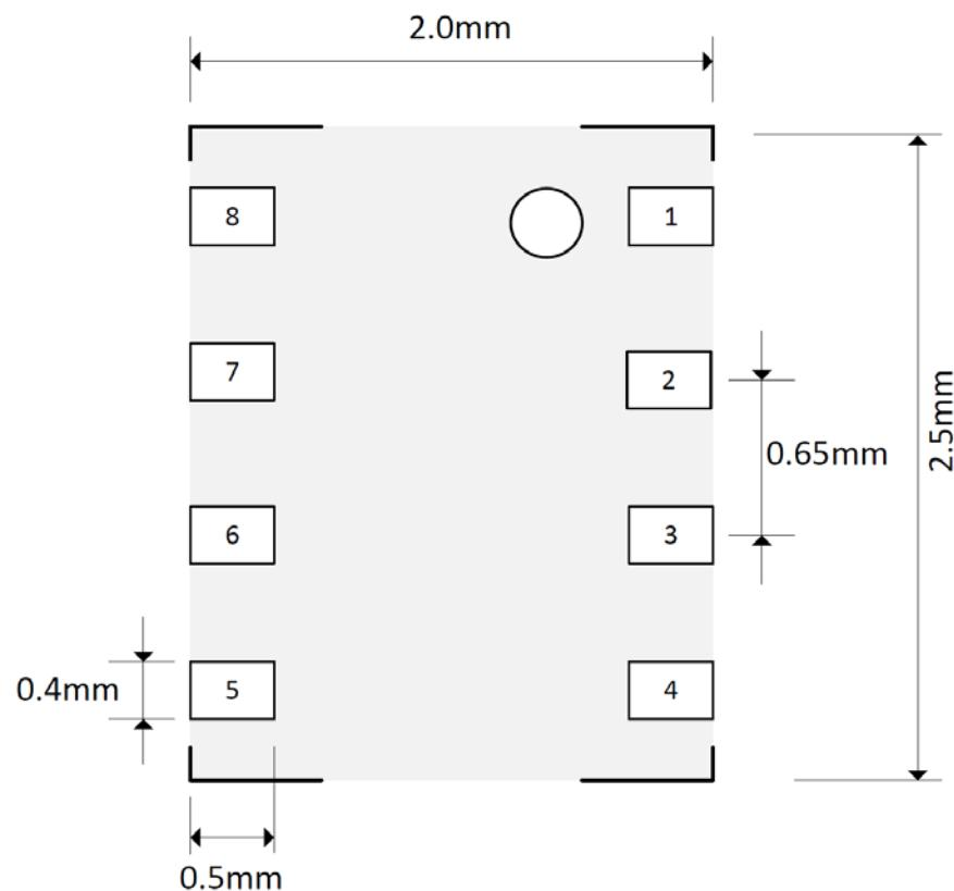
**Figure 12. ICP-10110 & ICP-10111 recommended PCB land pattern**
