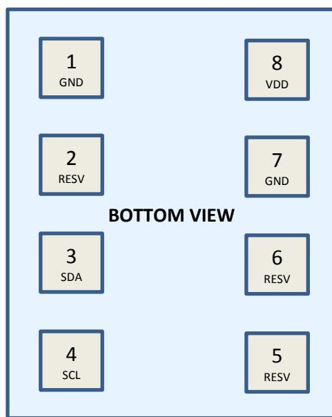
**Figure 3. Pin Out Diagram for ICP-10110 & ICP-10111 2 mm x 2.5 mm x 0.92 mm LGA**
