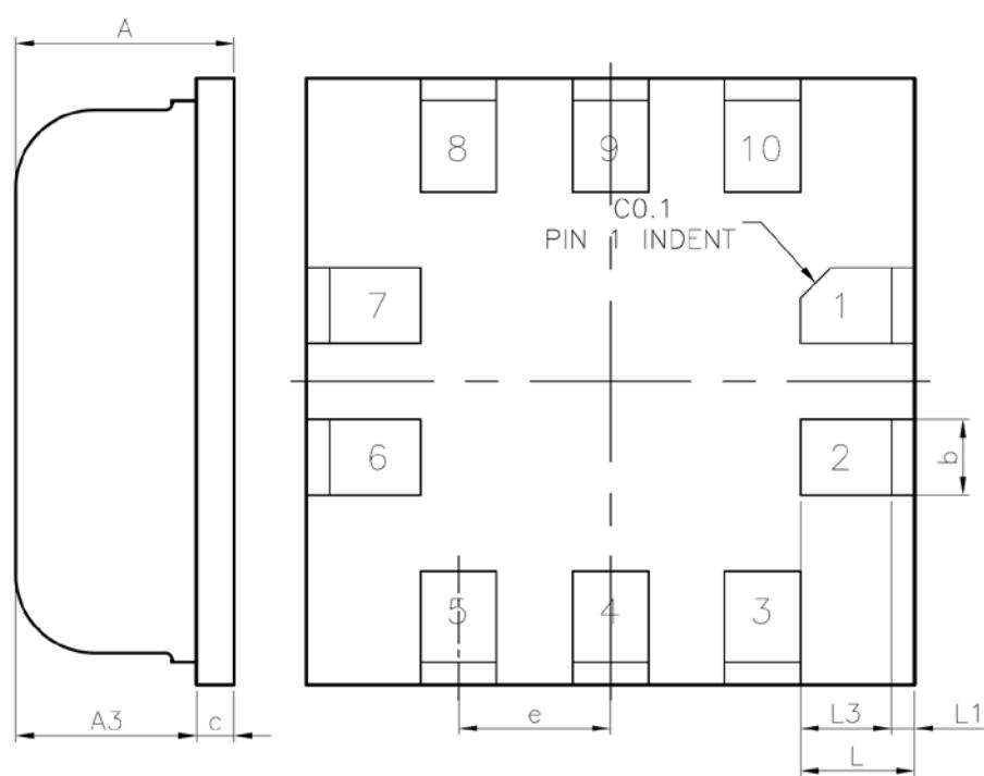
**Figure 9. ICP-10100 & ICP-10101 Package Diagrams**
