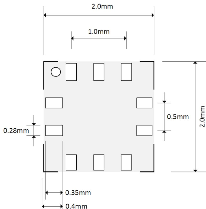
**Figure 10. ICP-10100 & ICP-10101 recommended PCB land pattern**
