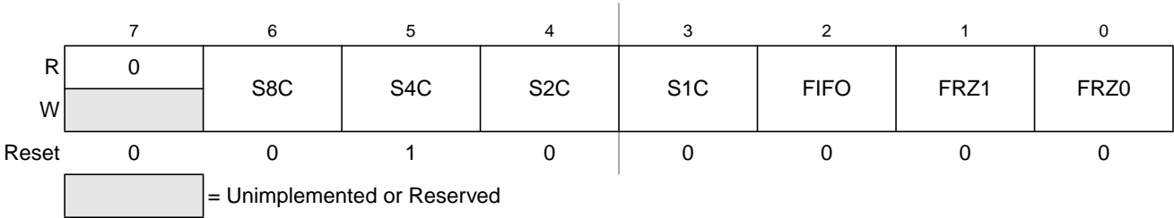
Figure 8-6. ATD Control Register 3 (ATDCTL3)
