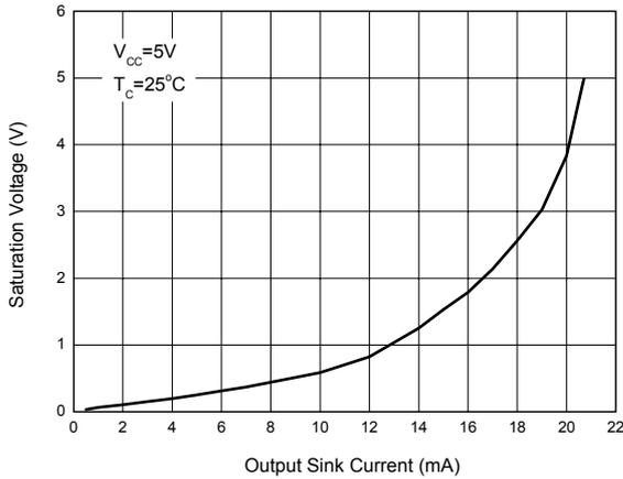
Figure 8. Saturation Voltage vs. Output Sink Current
