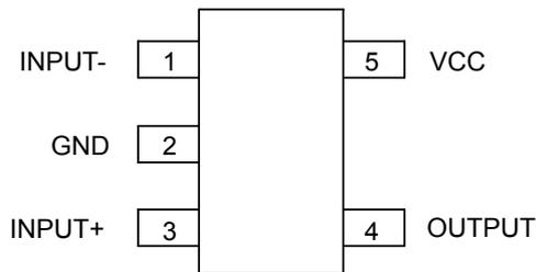
Figure 2. Pin Configuration of AS331 (Top View)
