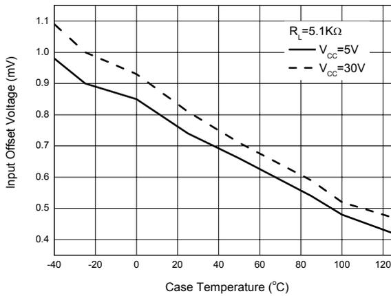
Figure 6. Input Offset Voltage vs. Case Temperature
