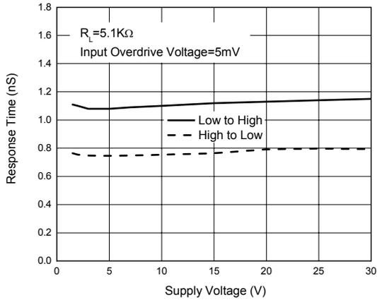
Figure 12. Response Time vs. Supply Voltage
