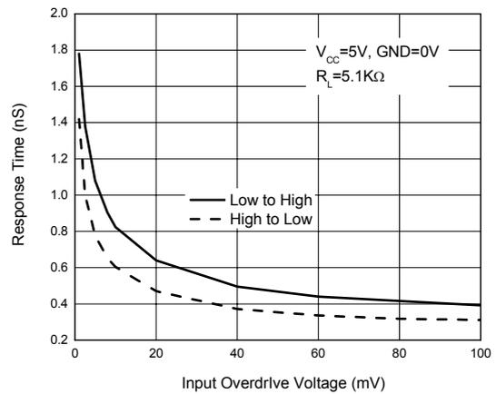
Figure 11. Response Time vs. Input Overdrive Voltage
