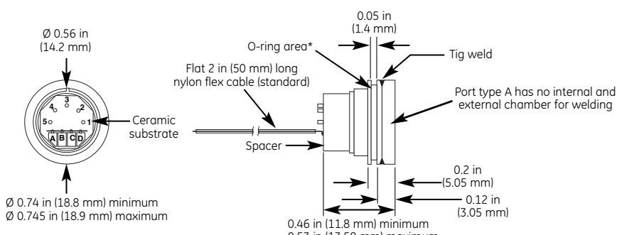
\*Uses o-ring 0.66 in ID x 0.039 in (16.76 mm x 1 mm) cross section.
