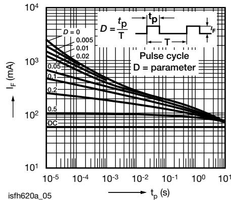
Fig. 6 - Permissible Pulse Handling Capability Forward Current vs.
