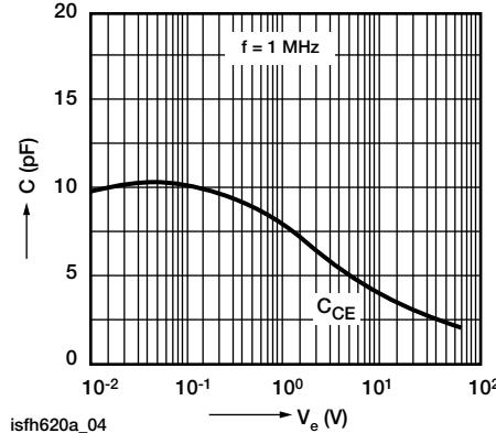
Fig. 5 - Transistor Capacitance (Typ.) vs. Collector Emitter Voltage
