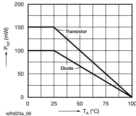
Fig. 7 - Permissible Power Dissipation vs. Ambient Temperature
