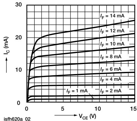
Fig. 3 - Output Characteristics (Typ.) Collector Current vs.
