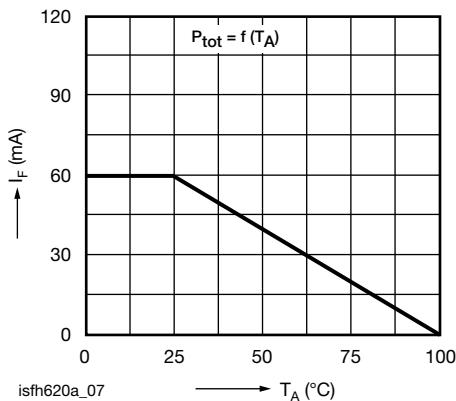
Fig. 8 - Permissible Diode Forward Current vs.
