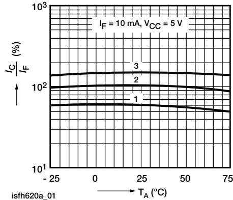
Fig. 2 - Current Transfer Ratio (CTR) vs. Temperature
