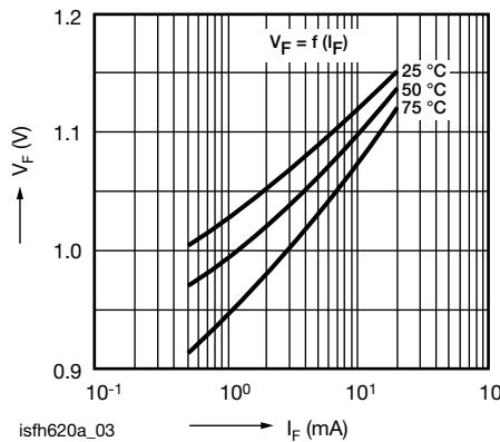
Fig. 4 - Diode Forward Voltage (Typ.) vs. Forward Current
