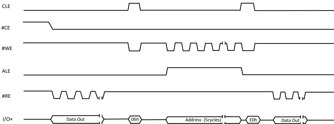
Figure 9-4 Two Plane Random Data Read (06h-E0h) Operation
