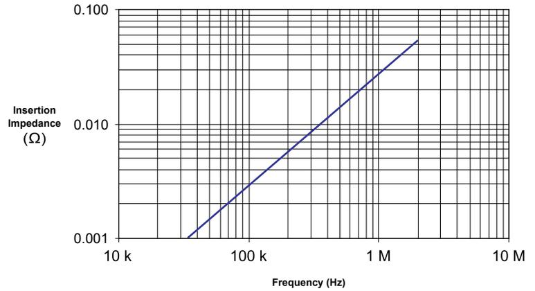
Insertion Impedance vs. Frequency
