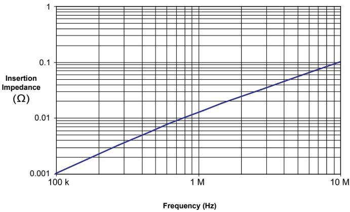
Insertion Impedance vs. Frequency\*
