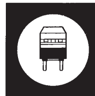
Stand-Off Lugs Minimize Solder-Creepage
