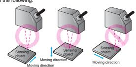
Install the Sensor as shown in the following if each sensing object greatly differs in color or material.
