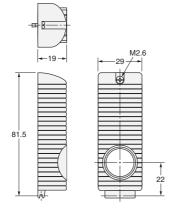
Note: 1. The cover is provided with a rubber bushing and cap to prevent the cable from being pulled out vertically.
