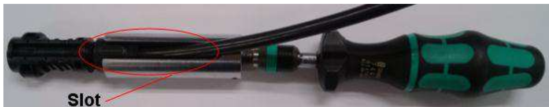
Figure 9 Tightening of the cable screw joint nut
