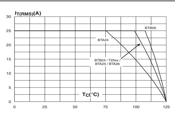
**Figure 3. D<sup>2</sup>PAK RMS on-state current versus ambient temperature (printed circuit board FR4, copper thickness: 35µm) (full cycle)**
