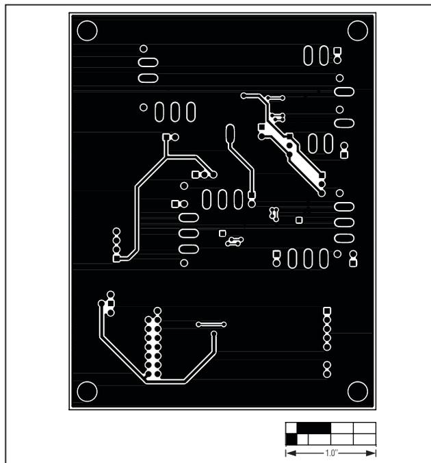
Figure 7. MAX5391L/MAX5391N EV Kit PCB Layout—Solder Side
