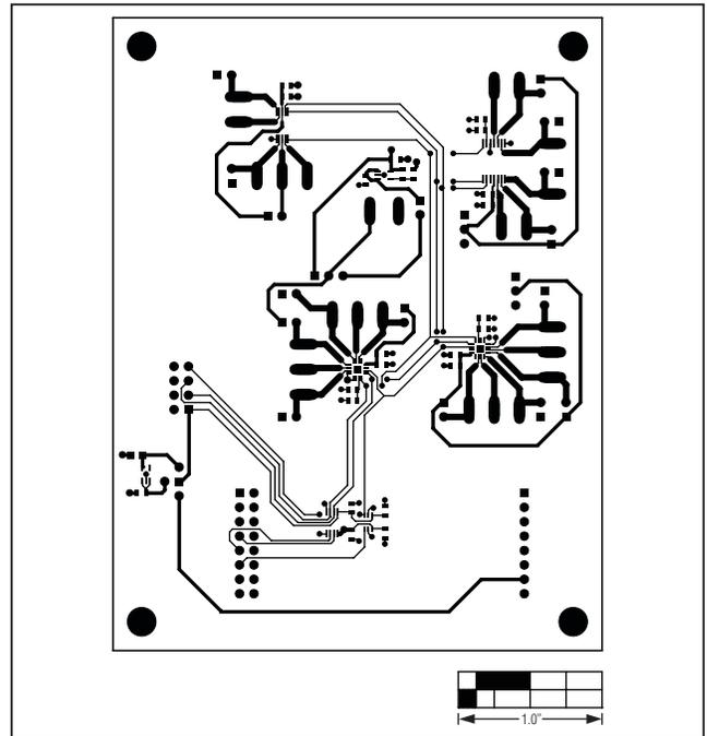
Figure 6. MAX5391L/MAX5391N EV Kit PCB Layout—Component Side
