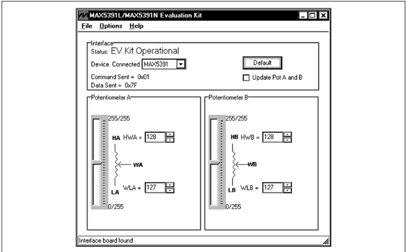
Figure 1. MAX5391L/MAX5391N Evaluation Kit Software Main Window
