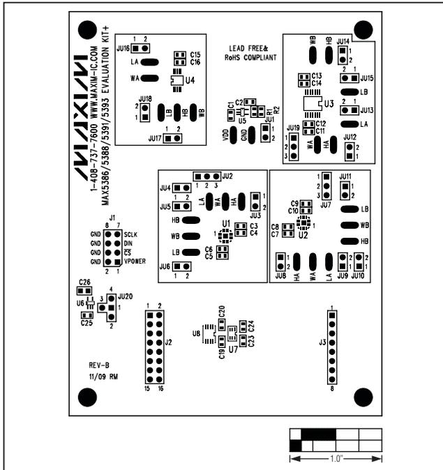
Figure 5. MAX5391L/MAX5391N EV Kit Component Placement Guide—Component Side
