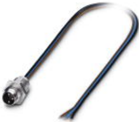
Sensor/actuator flush-type plug, 3-pos., M8, front/screw mounting, with M8 thread, with 0.5 m TPE litz wire, 3 x 0.25 mm 2
