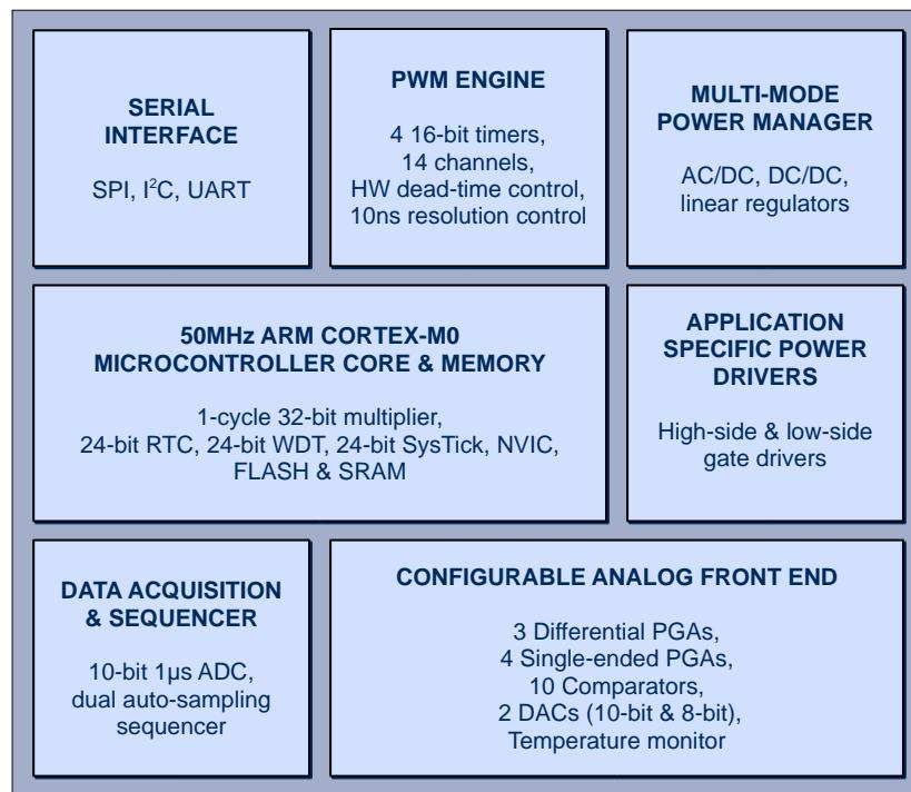
The PAC5225 is available in a 48-pin, 6x6 mm TQFN package. The PAC family includes a range of part numbers optimized to work with different targeted primary applications.
