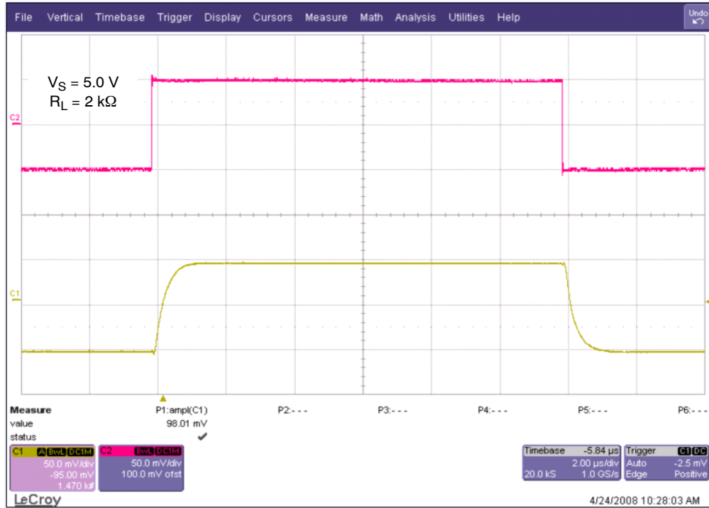
Figure 18. Small Signal Noninverting Response
