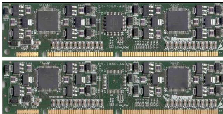
Figure 1: PoE PD67124 DIMM
