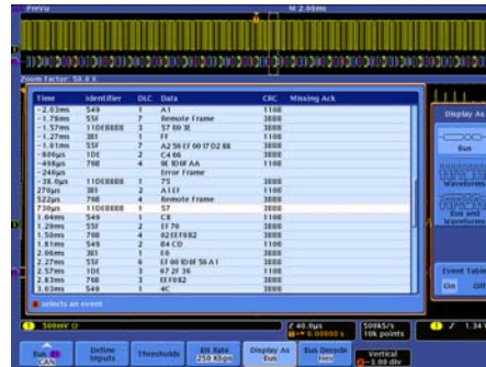
CAN event table display of bus content for easy comparison with software listings.
