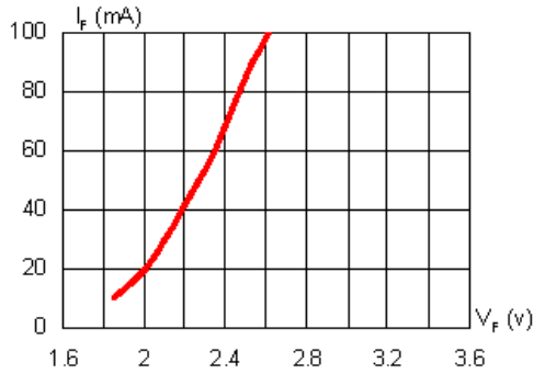
Fig.1 Forward Current vs. Forward Voltage
