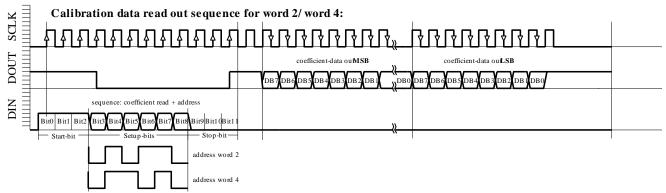
Fig. 6d: W2, W4 READING sequence
