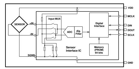
Fig. 1: Block diagram MS5536C
