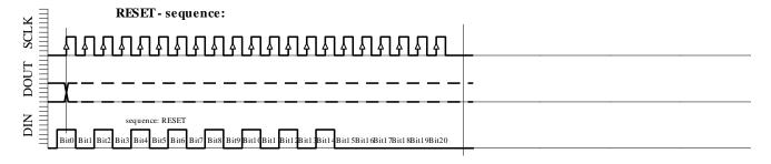
Fig. 6e: RESET sequence (21 bit)
