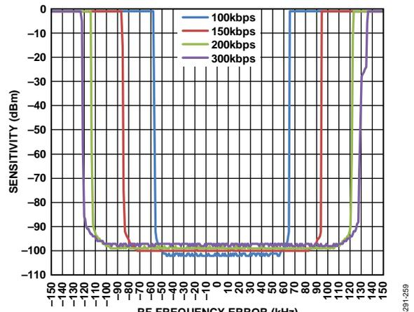
Figure 63. AFC On: Receiver Sensitivity (at PER = 1%) vs. RF Frequency Error, GFSK, 915 MHz, AFC Enabled ( $K_i = 7$ ,  $K_p = 3$ ), AFC Mode = Lock After Preamble, IF Bandwidth = 100 kHz (at 100 kbps), 150 kHz (at 150 kbps), 200 kHz (at 200 kbps), and 300 kHz (at 300 kbps), Preamble Length = 64 Bits
