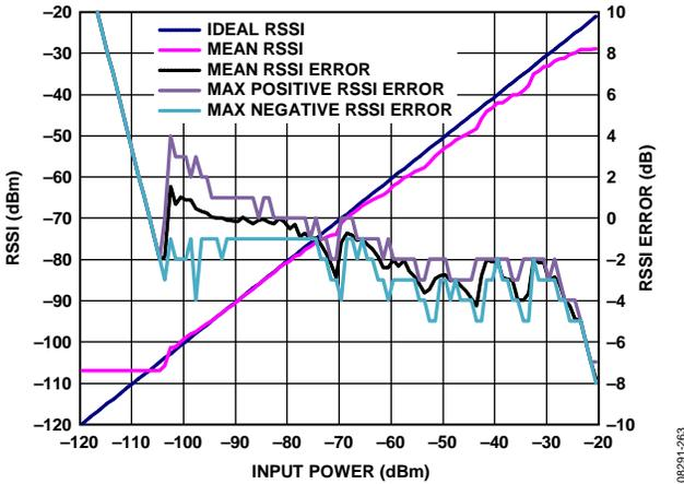
Figure 67. RSSI (via Automatic End of Packet RSSI Measurement) vs. RF Input Power, 868 MHz, GFSK, Data Rate = 300 kbps, Frequency Deviation = 75 kHz, IF Bandwidth = 300 kHz, AGC\_CLOCK\_DIVIDE = 15, 100 RSSI Measurements at Each Input Power Level
