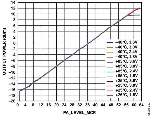
Figure 11. Differential PA at 433 MHz: Output Power vs. PA\_LEVEL\_MCR Setting, Temperature, and V<sub>DD</sub> (Minimum Recommended V<sub>DD</sub> = 2.2 V, 1.8 V Operation Shown for Robustness)
