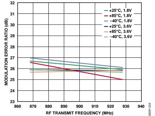
Figure 28. Modulation Error Ratio (MER) vs. RF Frequency, Temperature, and V<sub>DD</sub> at Modulation Index = 0.5 and Data Rate = 10 kbps
