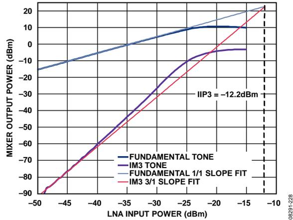
Figure 32. LNA/Mixer IIP3,  $V_{DD} = 3.0\text{ V}$ , Temperature =  $25^\circ\text{C}$ , RF Frequency = 915 MHz, LNA Gain = High, Mixer Gain = High, Source 1 Frequency = (915 + 0.4) MHz, Source 2 Frequency = (915 + 0.7) MHz
