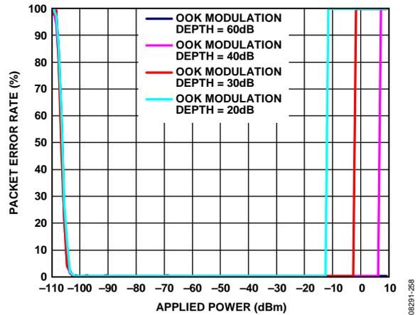
Figure 62. OOK Packet Error Rate vs. RF Input Power and OOK Modulation Depth, Data Rate = 19.2 kbps (Chip Rate = 38.4 kcps, Manchester Encoded), IF Bandwidth = 100 kHz,  $V_{DD}$  = 3.6 V, Temperature = 25°C, RF Frequency = 902 MHz, Preamble Length = 100 Bits
