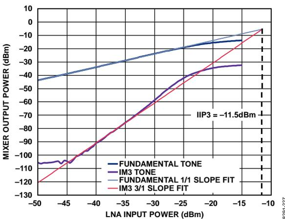
Figure 31. LNA/Mixer IIP3,  $V_{DD} = 3.0\text{ V}$ , Temperature =  $25^\circ\text{C}$ , RF Frequency = 915 MHz, LNA Gain = Low, Mixer Gain = Low, Source 1 Frequency = (915 + 0.4) MHz, Source 2 Frequency = (915 + 0.7) MHz
