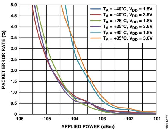
Figure 61. OOK Packet Error Rate vs. RF Input Power,  $V_{DD}$  and Temperature, Data Rate = 19.2 kbps (Chip Rate = 38.4 kcps, Manchester Encoded), IF Bandwidth = 100 kHz,  $V_{DD}$  = 3.6 V, Temperature = 25°C, RF Frequency = 902 MHz, Preamble Length = 100 Bits (Minimum Recommended  $V_{DD}$  = 2.2 V, 1.8 V Operation Shown for Robustness)
