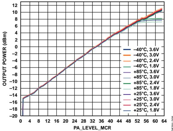
Figure 13. Differential PA at 915 MHz: Output Power vs. PA\_LEVEL\_MCR Setting, Temperature, and V<sub>DD</sub> (Minimum Recommended V<sub>DD</sub> = 2.2 V, 1.8 V Operation Shown for Robustness)
