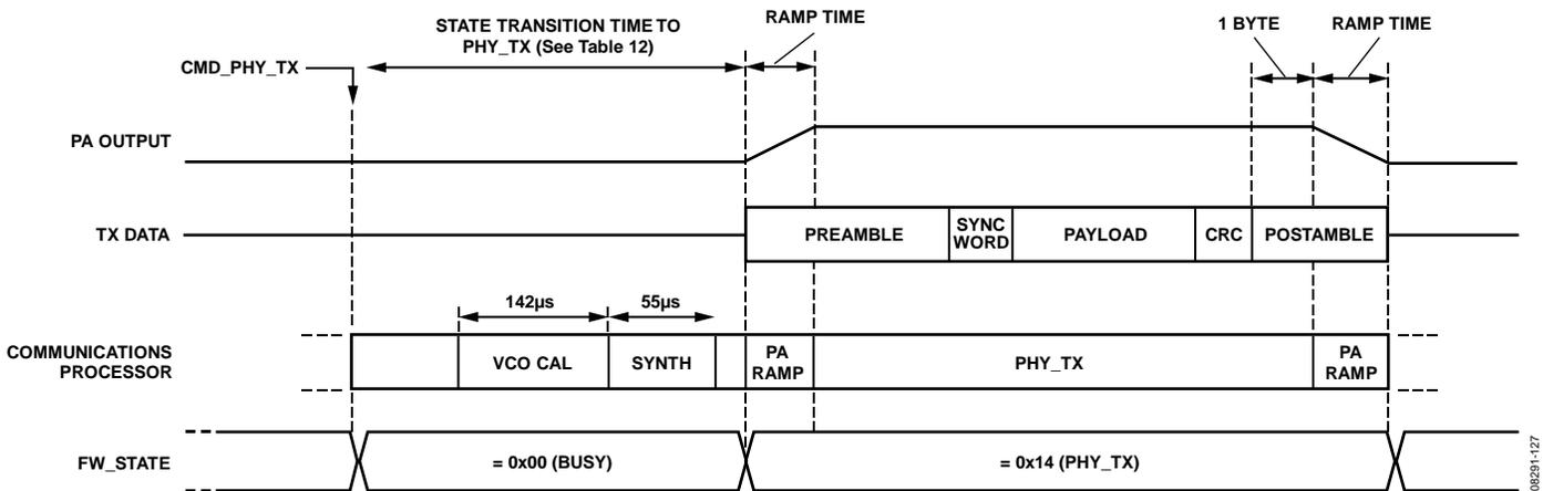
Figure 79. Transmit Packet Timing
