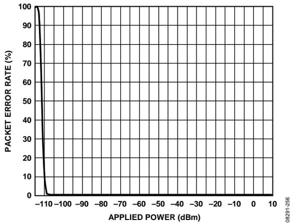
Figure 60. OOK Packet Error Rate vs. RF Input Power, Data Rate = 2.4 kbps (Chip Rate = 4.8 kcps, Manchester Encoded), IF Bandwidth = 100 kHz,  $V_{DD}$  = 3.6 V, Temperature = 25°C, RF Frequency = 902 MHz, Preamble Length = 100 Bits
