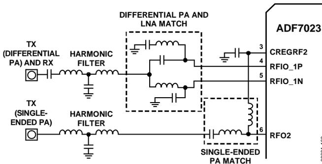
Figure 116. Matching Topology for Transmit Antenna Diversity
