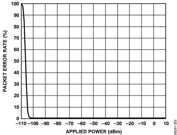
Figure 59. OOK Packet Error Rate vs. RF Input Power, Data Rate = 19.2 kbps (Chip Rate = 38.4 kcps, Manchester Encoded), IF Bandwidth = 100 kHz,  $V_{DD}$  = 3.6 V, Temperature = 25°C, RF Frequency = 902 MHz, Preamble Length = 100 Bits
