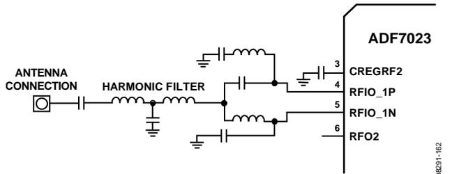
Figure 115. Combined Differential PA and LNA Match
