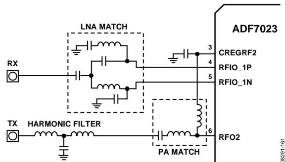
Figure 114. Separate Single-Ended PA and LNA Match
