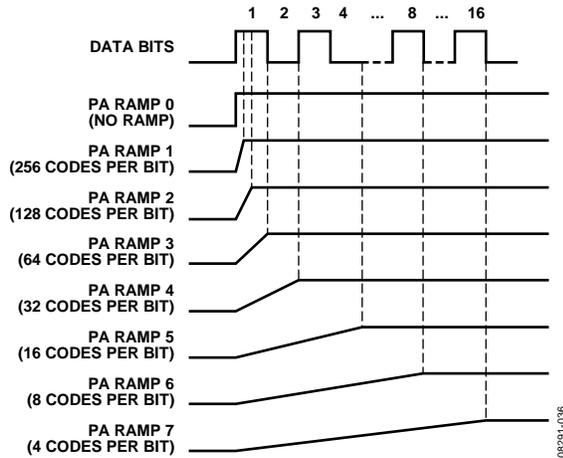
Figure 108. PA Ramp for Different PA\_RAMP Settings
