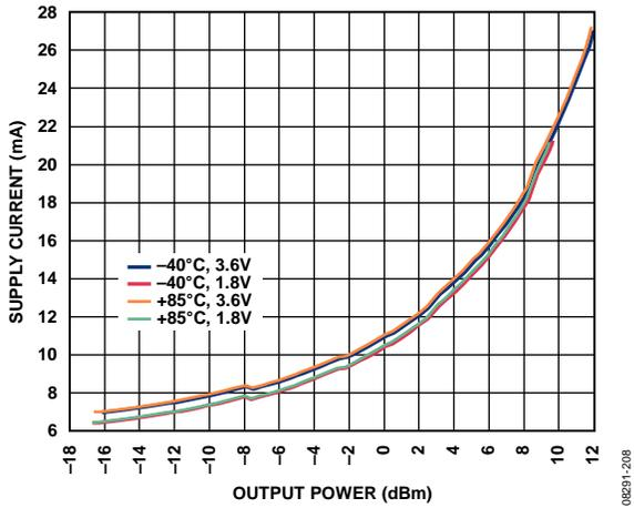
Figure 12. Differential PA at 433 MHz: Supply Current vs. Output Power, Temperature, and V<sub>DD</sub> (Minimum Recommended V<sub>DD</sub> = 2.2 V, 1.8 V Operation Shown for Robustness)
