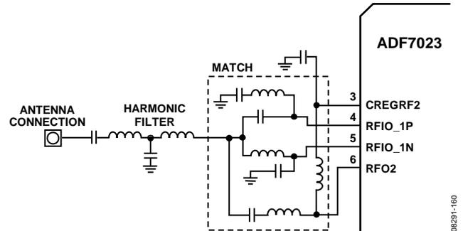
Figure 113. Combined Single-Ended PA and LNA Match
