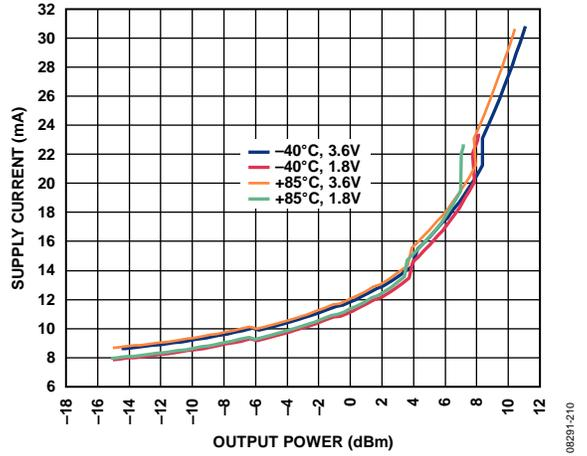
Figure 14. Differential PA at 915 MHz: Supply Current vs. Output Power, Temperature, and V<sub>DD</sub> (Minimum Recommended V<sub>DD</sub> = 2.2 V, 1.8 V Operation Shown for Robustness)
