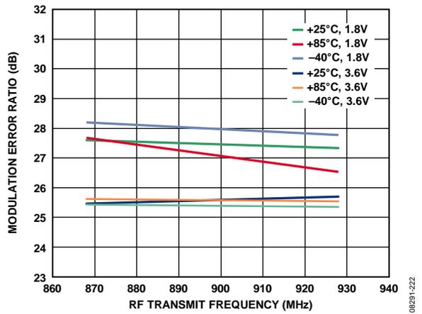
Figure 26. Modulation Error Ratio (MER) vs. RF Frequency, Temperature, and V<sub>DD</sub> at Modulation Index = 1 and Data Rate = 10 kbps (Minimum Recommended V<sub>DD</sub> = 2.2 V, 1.8 V Operation Shown for Robustness)
