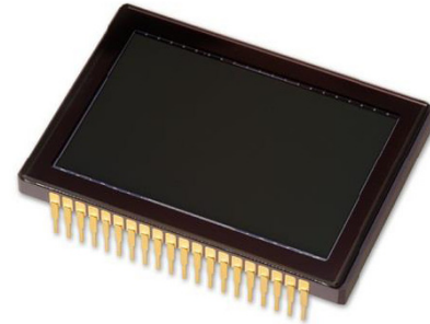
Figure 1. KAI-11002 Interline CCD Image Sensor
