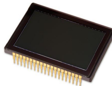
Figure 1. KAI-11002 Interline CCD Image Sensor
