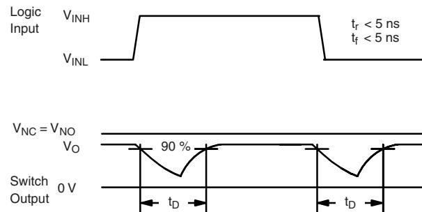
Figure 2. Break-Before-Make Interval
