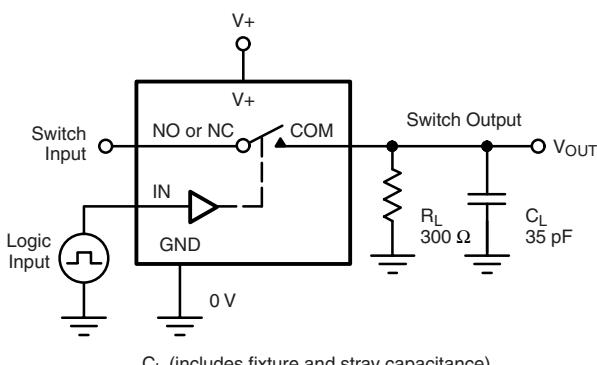
$$V_{OUT} = V_{COM} \left( \frac{R_L}{R_L + R_{ON}} \right)$$
