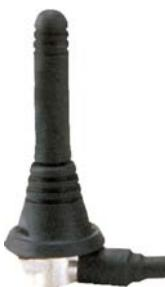
Designed for permanent mounting through a metal surface such as an automobile roof or trunk, the compact RMS Series offers excellent performance in a durable and unobtrusive housing. The antenna may be operated at either or both of two frequency bands. It is supplied with 14.1 feet (4.3m) of RG-58 cable and can be terminated in a standard SMA, Part 15 compliant RP-SMA or a TNC connector.
